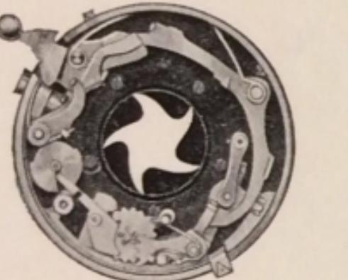
Note the unusual simplicity of mechanical parts. The little wheel shown at the bottom is not a gear but an escapement wheel that makes only a partial revolution.
