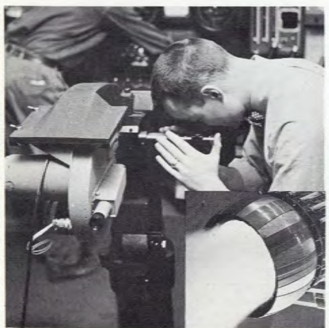
Close-up view of combustion process within the afterburner of advanced jet engine test.
