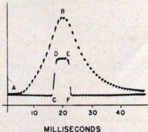
*ALL RAPAX Shutter speeds and the delayed action of the synchronizer and the duration of contacts are checked in milliseconds on the GE Time-Interval Meter.*
