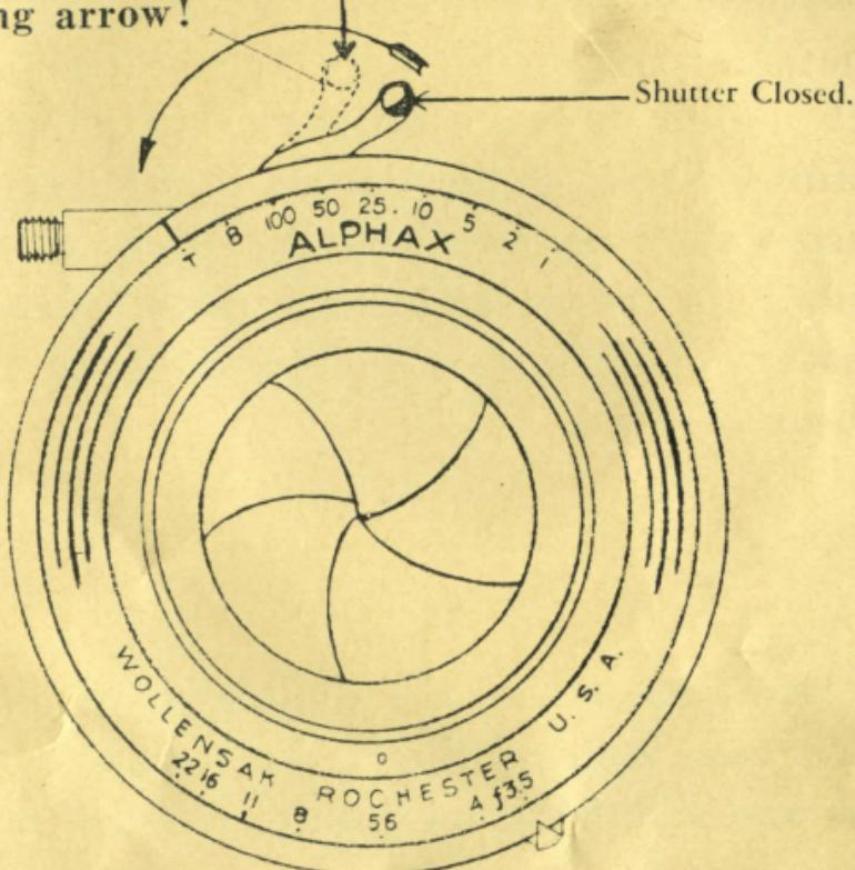
B or BULB Exposure is used for making exposures of prolonged duration. Set the speed indicator to "B" and trip the release lever, or
