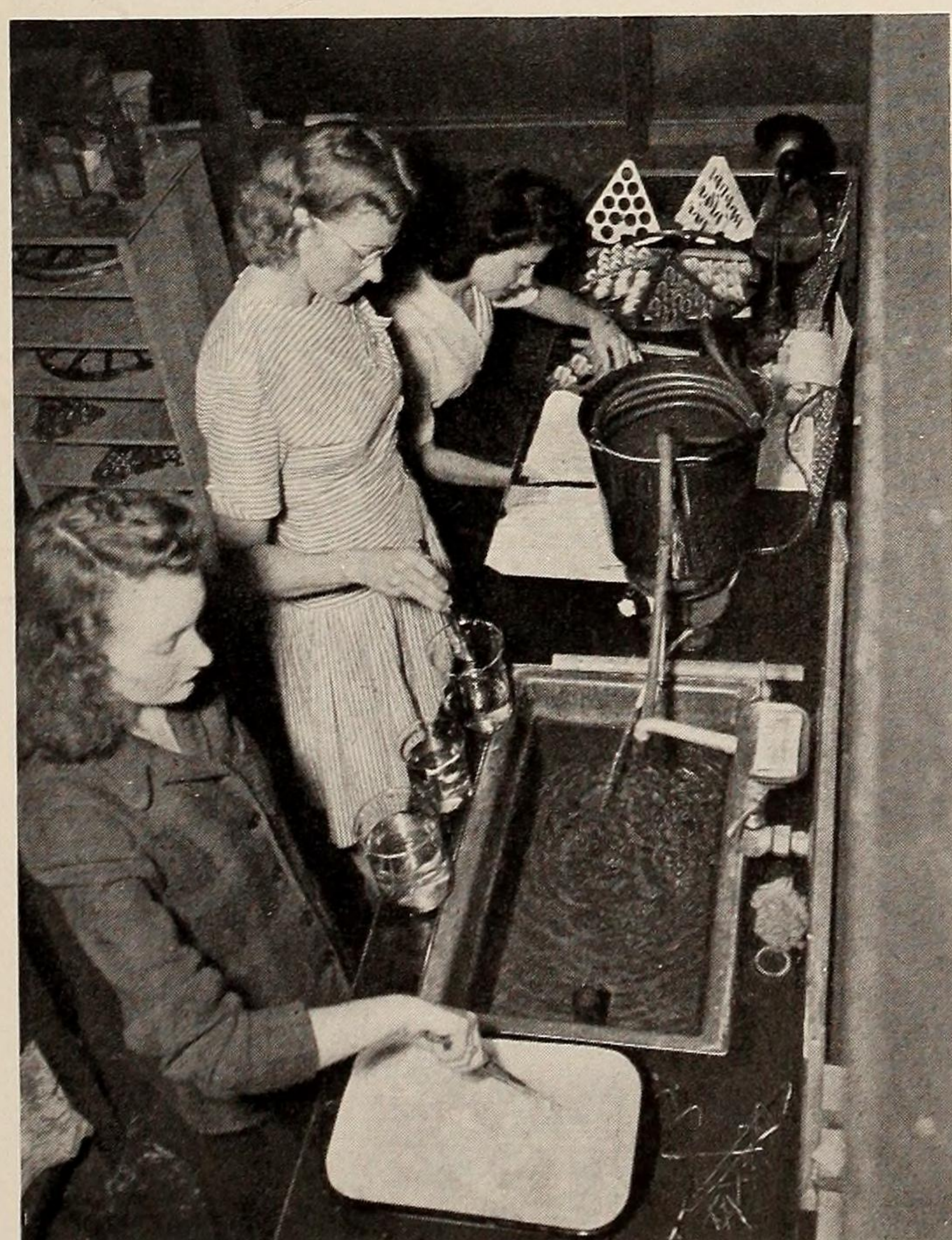
• Fig. 2. The dust free, properly air conditioned laboratory of the Wollensak Optical Company makes cleaning lenses a routine.
